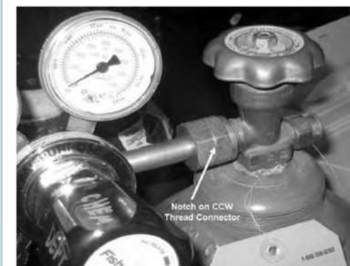
FIGURE 5.3.1.3 Notch in Connecting Nut Indicating CCW Thread. For most normal gases the CGA connector attaches clockwise (CW), but for flammable gases the CGA connector attaches counterclockwise (CCW).
