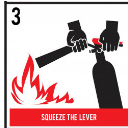
3. S queeze the handle to begin the discharge
